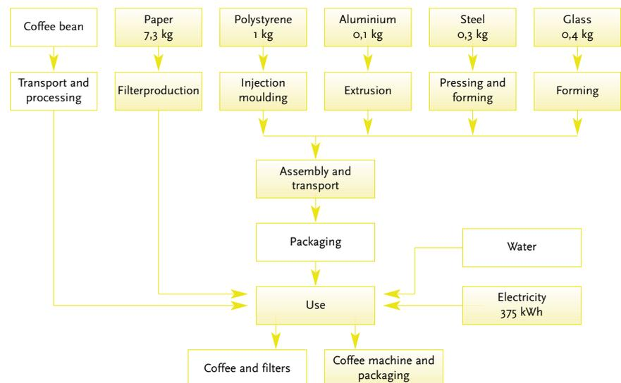
Figure 3: Process tree of a simplified coffee machine model with amounts and assumptions. White boxes are not included in the analysis.
