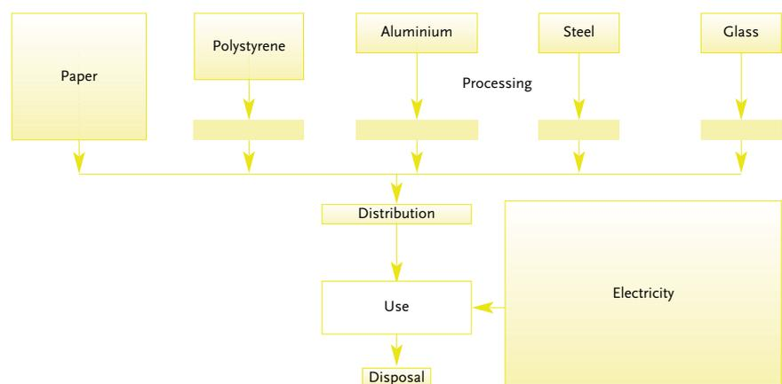
Figure 4: The coffee machine process tree, where the size of the process blocks is proportional to the relative importance of the process.
