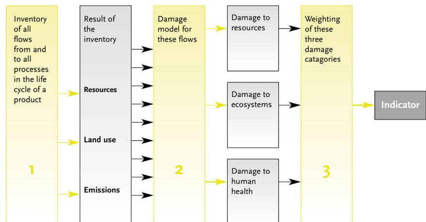
Figure 6: General procedure for the calculation of Eco-indicators. The light coloured boxes refer to procedures, the dark coloured boxes refer to intermediate results.
