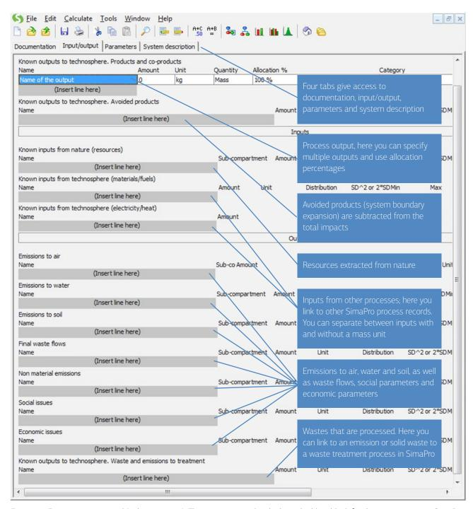
Figure 14: Empty process record (only upper part). This process record is the basic building block for the process trees in SimaPro.
