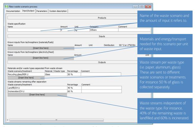
Figure 21: A waste scenario is used to split a waste stream. Splitting can be done per waste type or in a generic way.
