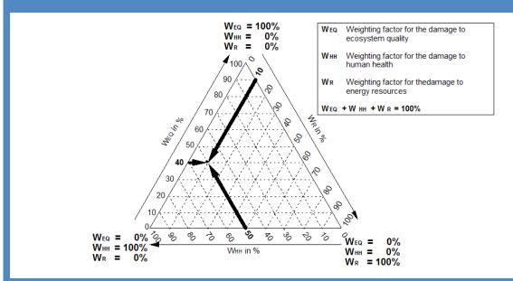
Figure 8: The mixing triangle: The marked weighting point is positioned where human health is weighted 50%, ecosystem quality 40% and resources 10%. This weighting point is defined as the point where the lines cross; the lines are drawn starting from the desired weighting factor and parallel to the axis which equals zero for that factor (based on Hofstetter 1999).
