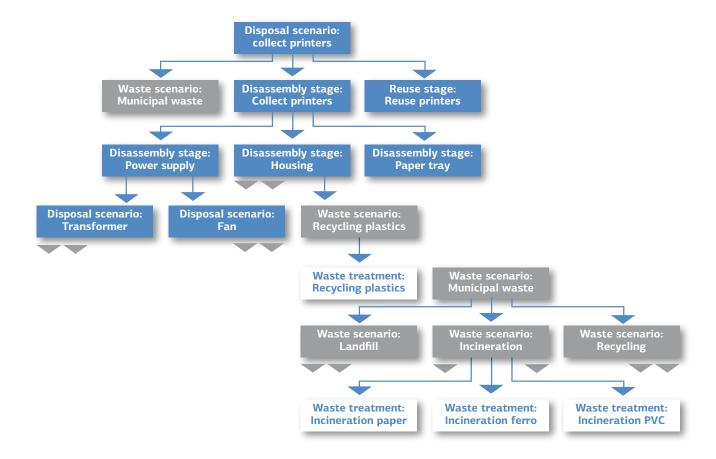
Figure 23: A disposal scenario specifies how products are distributed over different end-of-life options, such as disassemblies, reuse and waste scenarios. A disassembly specifies how products are split up in different components and to which destinations these are sent to.
