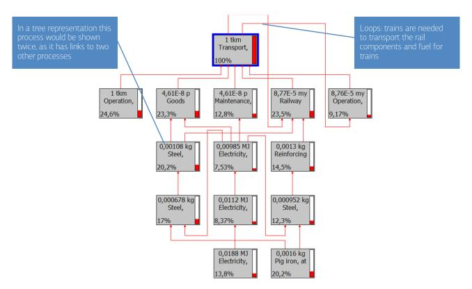
Figure 16: Example of a network representation that contains loops. Only the most relevant of in total 1999 processes are displayed.
