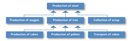
Figure 15: Schematic overview of how processes are linked to form a process tree structure. In this case unit processes are used that describe a single process step, which provides the highest transparency.
