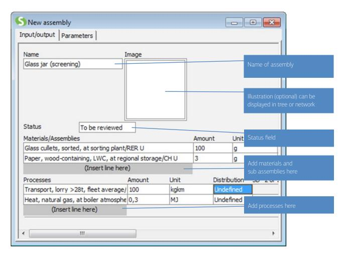
Figure 17: An example of a product stage, in this case the assembly.
